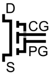
Figure 1: Symbol of a 2-Gate RFET.
